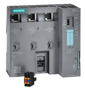
SIMATIC DP, IM151-8 PN/DP CPU FOR ET200S, 192 KB WORKING MEMORY, INT. PROFINET INTERFACE (WITH THREE RJ45 PORTS) AS IO-CONTROLER, W/O BATTERY MMC REQUIRED
