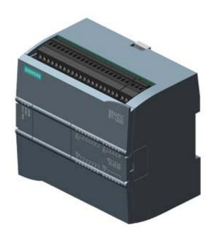
SIMATIC S7-1200, CPU 1214C, COMPACT CPU, DC/DC/DC, ONBOARD I/O: 14 DI 24V DC; 10 DO 24 V DC; 2 AI 0 - 10V DC,
