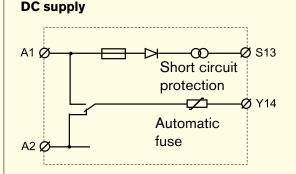
The RT9 should be supplied with +24 V on A1 and 0 V on A2.
