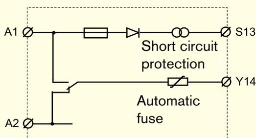
The RT9 should be supplied with +24 V on A1 and 0 V on A2.
