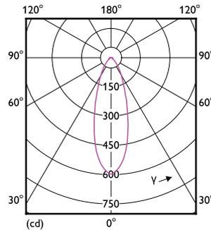
LEDspots Corepro SLR 4W PAR16 GU10 830 36D-LDD
