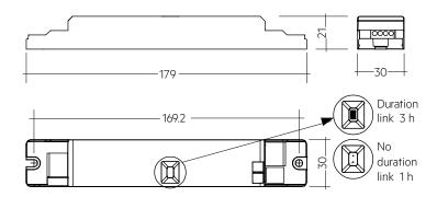
Note: Supply of control gear with duration link in 3 hours position. Remove duration link for duration of 1 h. Duration link must be set before battery and mains connection.
