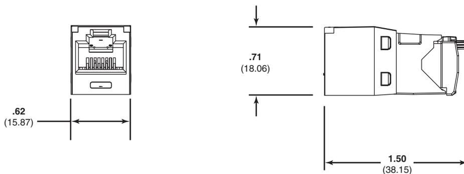
Dimensions are in inches (Dimensions in parenthesis are metric)
